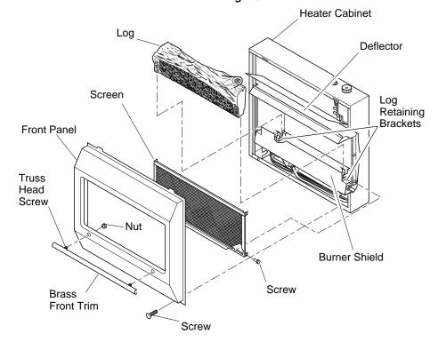
Figure 4 - Assembling Heater
